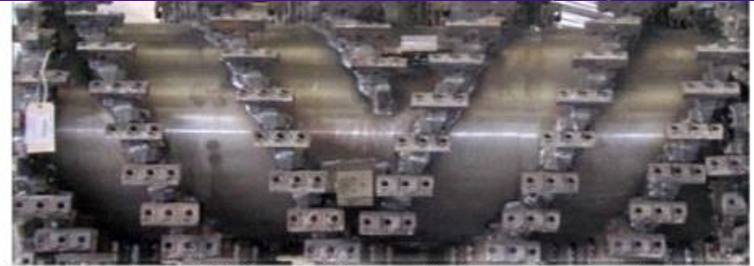
A micro-milling drum with 3 times (est.) more bits than a standard drum (Courtesy of Keystone Engineering)
